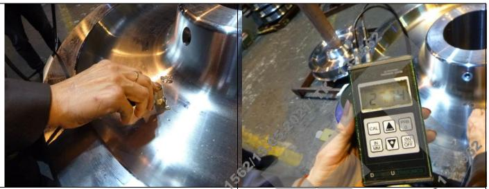
Photo 37 Web thickness measurement
